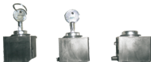
b. Two locks and one key: two circuit breakers are equipped with two identical locks and one key, and only one circuit breaker is allowed to be switched on
