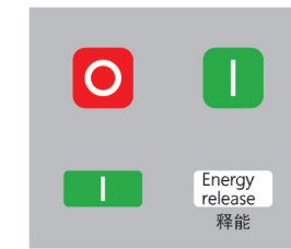
断路器合闸且无储能状态 Circuit breaker switched on and no energy storage
