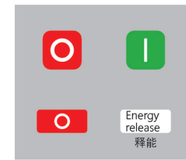
断路器断开且无储能状态 Circuit breaker is disconnected and no energy storage
